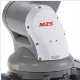
Stopper cover for reducing clamping risk
