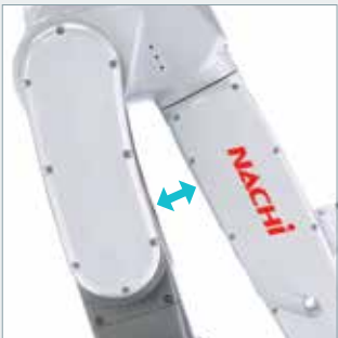
Offset arm shape for reducing clamping risk
